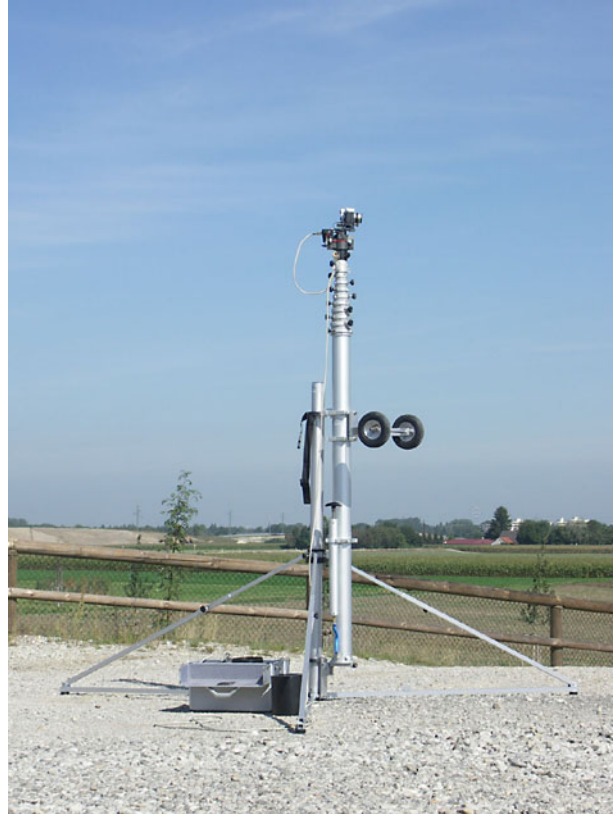
PT 150 installed into the tripod base with Remote Control 2 Zoom (remote camera control) prior to the extension of the tubes.
